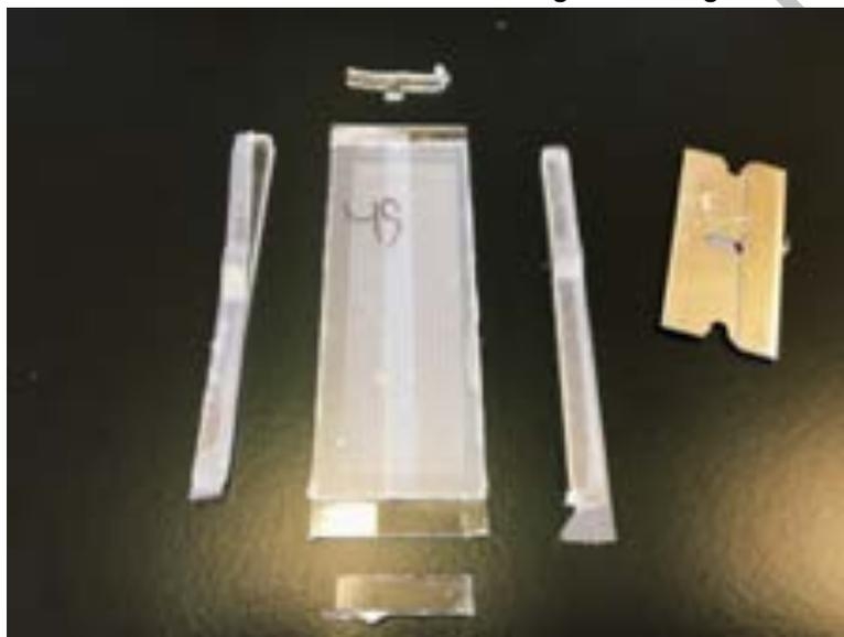
2. Use scotch tape to remove excess PDMS from the surface of the array and the glass slide.
